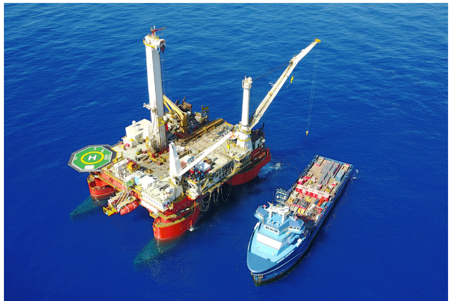
Q4000 semisubmersible well intervention unit.
