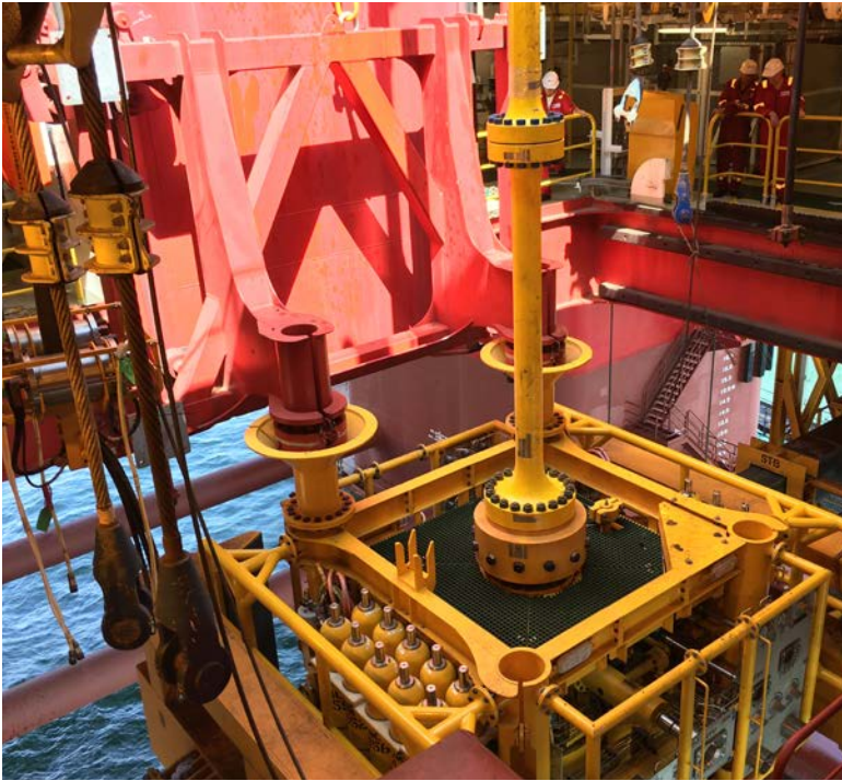
A single 10-week-long deployment of the proprietary intervention riser system across four subsea well hops efficiently enabled achievement of workover objectives on all five wells.
