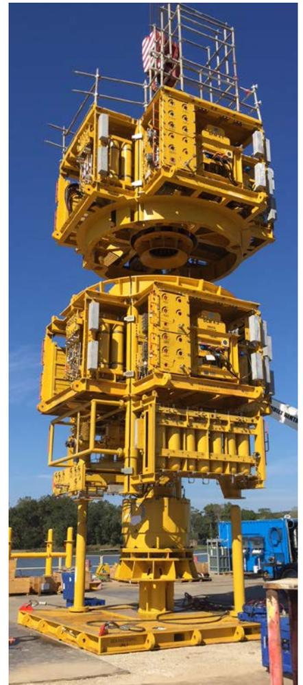
*The proprietary 15,000-psi intervention riser system was mobilized and demobilized much quicker and more cost-effectively than a conventional drilling rig.*
