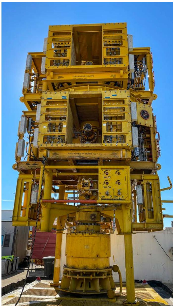
*The 15,000-psi intervention riser system streamlined access to subsea wells and was fitted with 33 directional control valves.*
