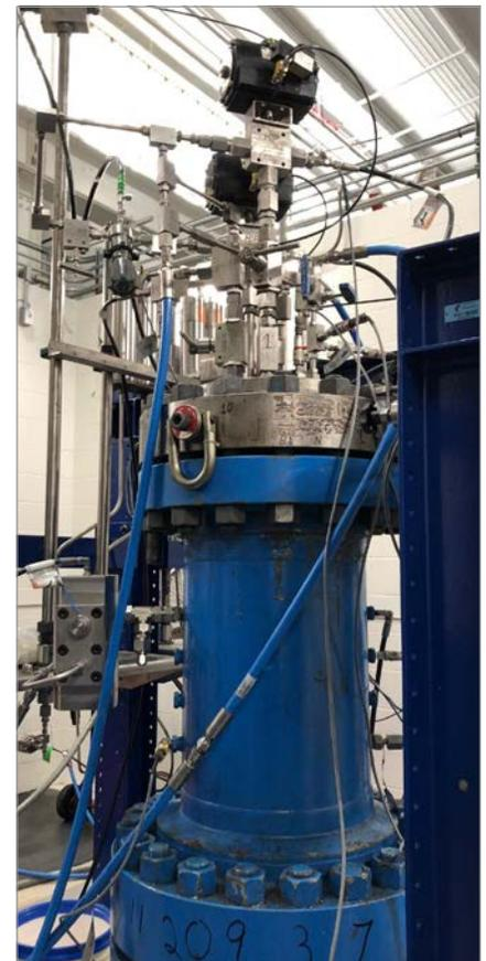
*The improved subsea directional control valve underwent extensive qualification testing that stressed it beyond the required operating envelope.*
